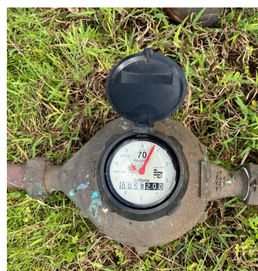
Figure 2: Water meter used to measure amount of water in control & CropManage plots
