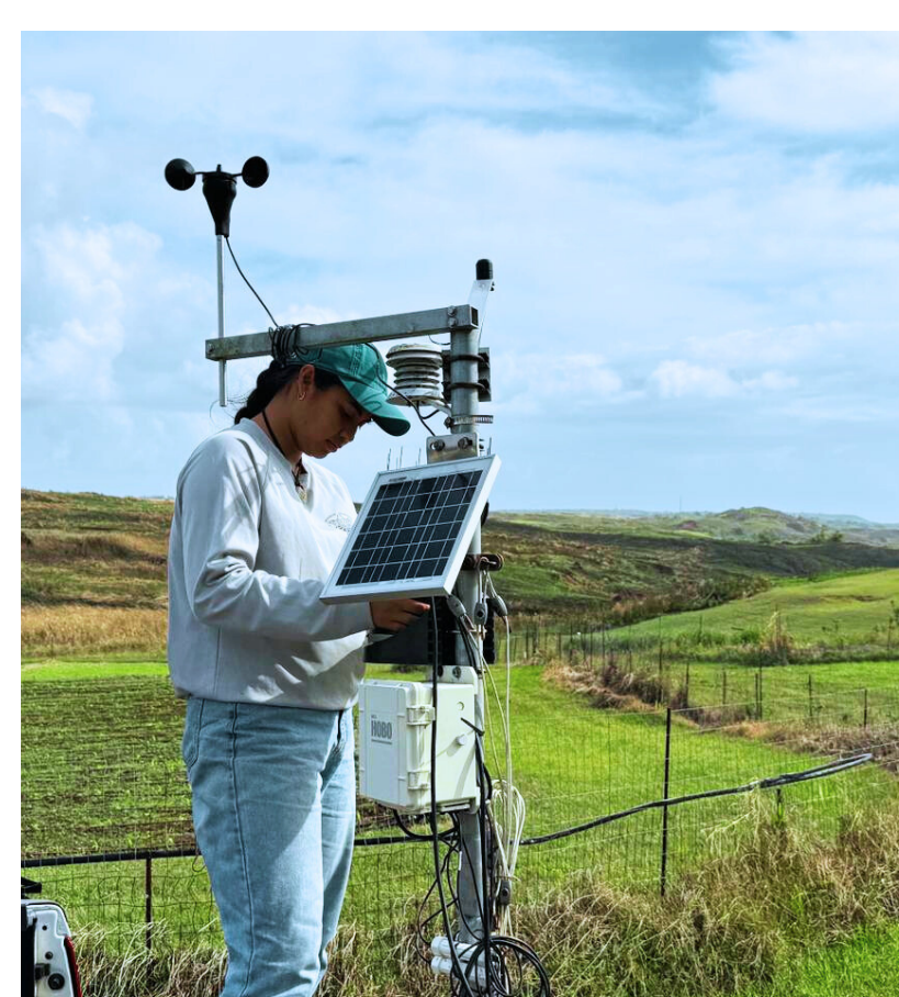
Figure 1: Set-up of weather station at Ija Research Experiment Station
