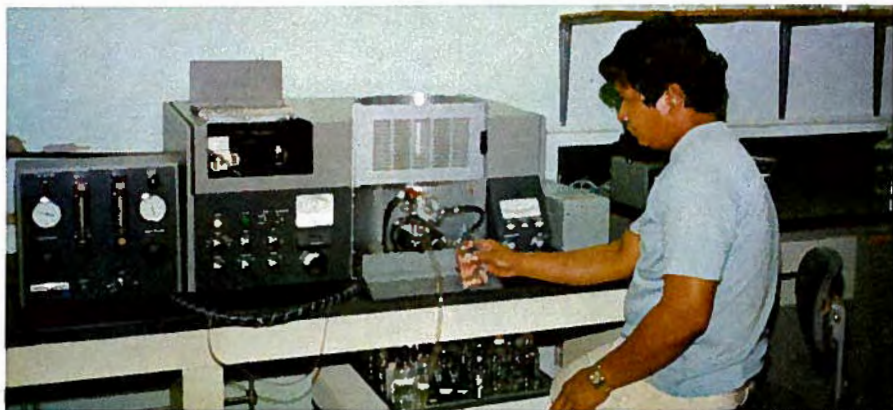
The AES Soil Research and Testing Laboratory has a Perkin-Elmer 305B Atomic Absorption Spectrophotometer (shown here with Chemist Joe Cruz).
